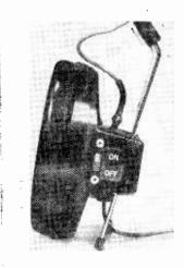
When the built-in amplifier is turned off, the headset can be used as standard hi-fi phones for just about any purpose.
